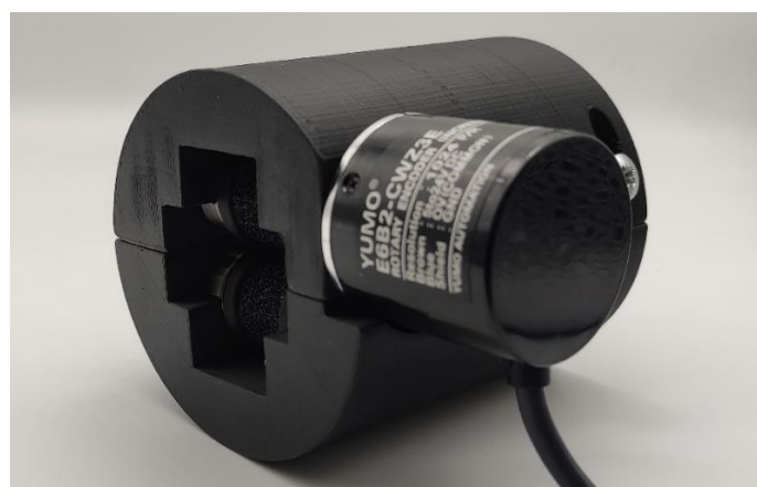
Figure 21: Assembled 3D Printed Tether Encoder Casing
